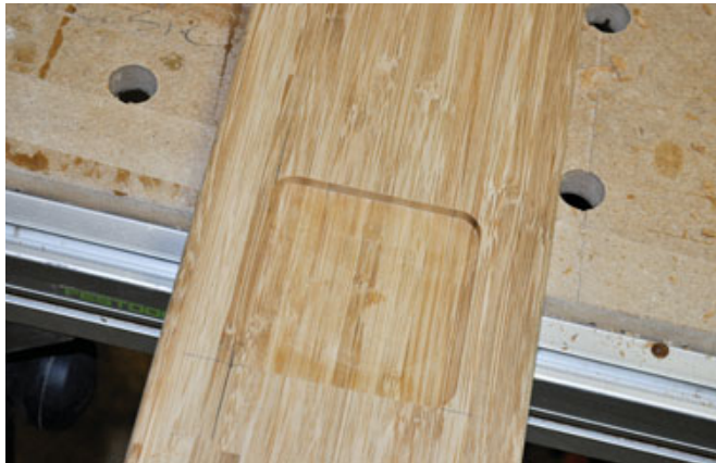
Figure 13. Router bits make radius corners. Square them with a chisel, or rout the same radius on the corners of the male piece, using a roundover bit.
