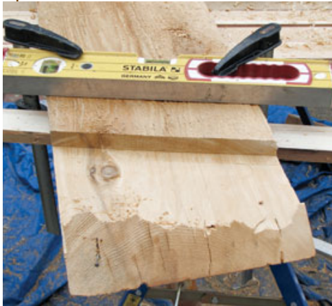
Figure 16. Leave the workpiece a little long, and work inward as you cut a half-lap joint.
