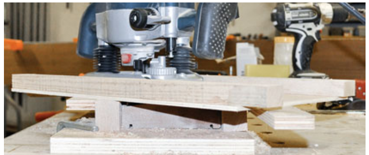
Figure 20. A second jig atop the first guides the router to make an angled lap cut on profiled stock.
