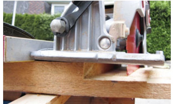
Figure 17. Adjust the straightedge as needed to guide a circular saw in cutting the work to length.
