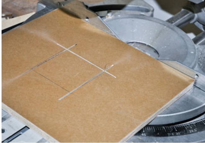
Figure 12. Make a mortise template from material that's slightly deeper than the distance the bushing extends from the router base.
