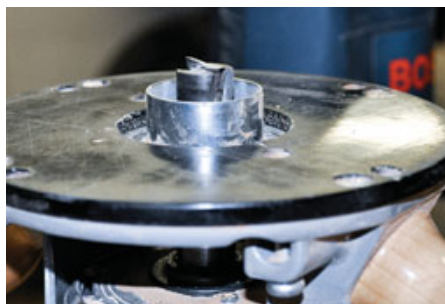
Figure 11. Guide bushings ride on templates, guiding straight bits for cuts such as mortises.
