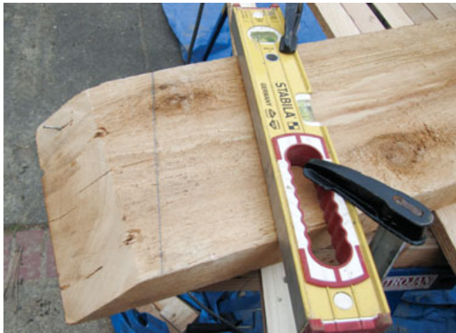
Figure 14. The simplest of router jigs can be a straightedge clamped to the workpiece.
