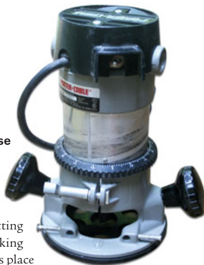
Figure 2. The plunge router's release lever allows the motor and bit to move up and down. Depth of cut can be preset.
