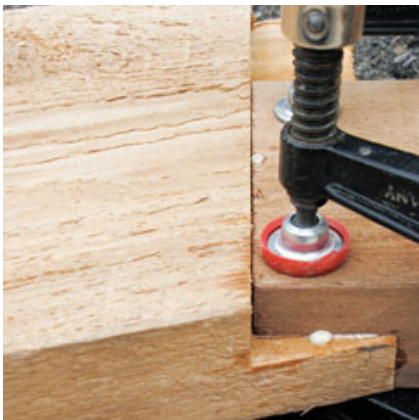
Figure 18. Glue and clamp a lap joint together.
