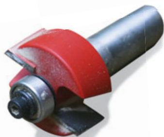
Figure 5. The bearing on a rabbet bit is smaller than the cutter diameter.
