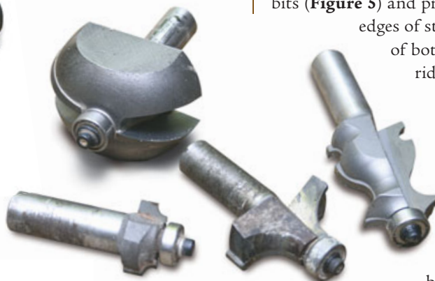
Figure 6. Profile bits shape material into quarter rounds, ogees, angles, and pretty much any pattern you can imagine.
