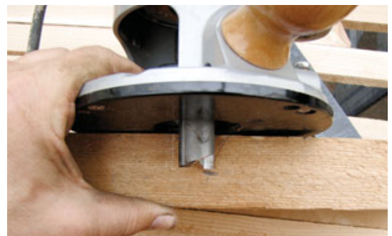
Figure 15. Hold the router in place to set the depth of cut for half-lap joints.
